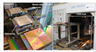
Fig. 1. Test setup: Left: Clamping of the sample sheets; Right: View into the vacuum chamber of the K30 (© Fraunhofer IPT)
